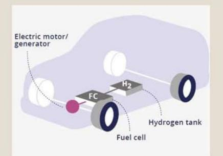
Fuel cell electric vehicles use a fuel cell to create on-board electricity, generally using compressed hydrogen and oxygen from the air.
