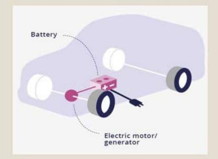
Battery electric vehicles are powered by an electric motor and battery with plugin charging.
