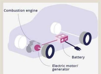
Plug-in hybrid electric vehicles have a conventional (petrol/diesel) engine complemented with an electric motor/battery with plug-in charging.
